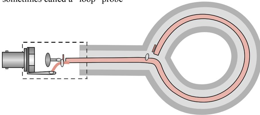
This probe would be improved with a CM choke or ferrite toroid.
