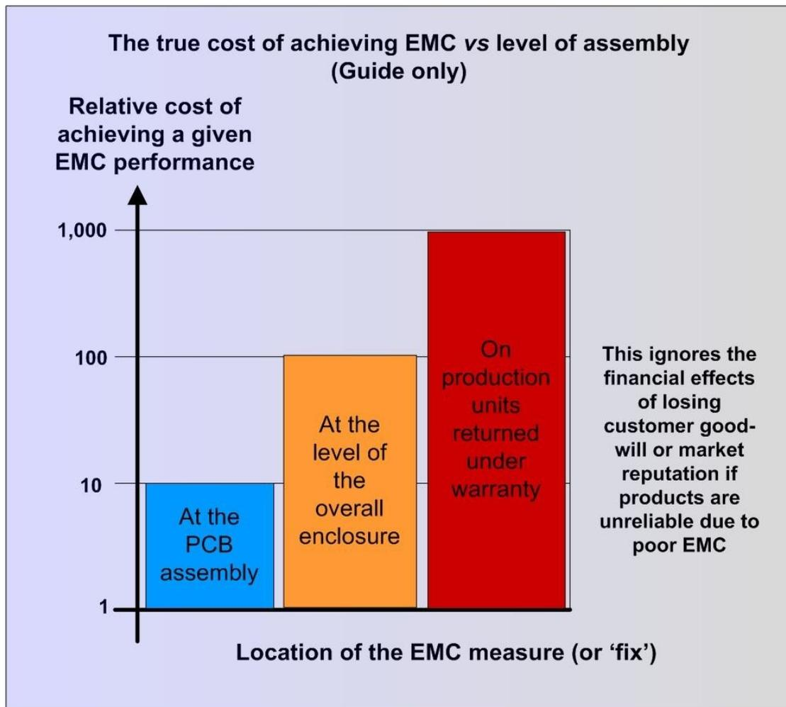
From the graph we can conclude that it is likely to be about a thousand times more costly to rectify a malfunction in equipment returning from the field than at the initial design stage.
