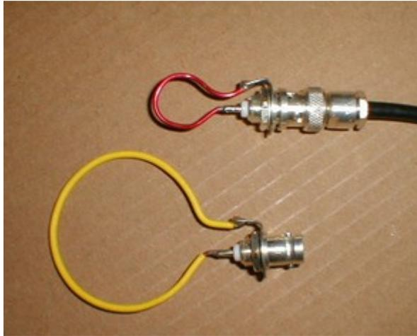
A rectangular probe can be more convenient for testing flat items
